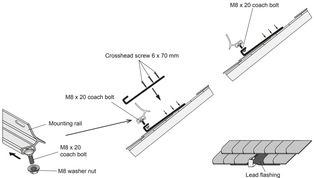
**CAUTION** Distribute all supplied double-ended screws evenly over the width of the collector array to spread the loads applied.
