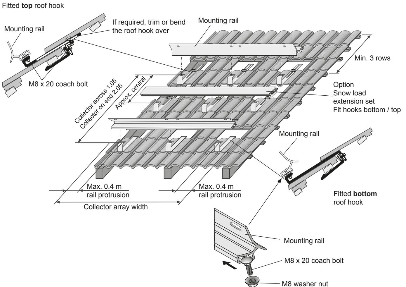
**CAUTION** Distribute all roof hooks supplied evenly over the width of the collector array to spread the loads applied. For this, position the roof hooks as near to the rafters as possible.
